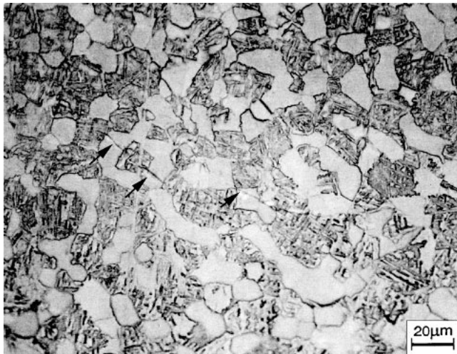
Fig. 9 Replicas of crack initiation site for material with bimodal forged microstructure ( R = 0.1 , \sigma_{\max} = 620 MPa, n = 1,990,000 cycles)
